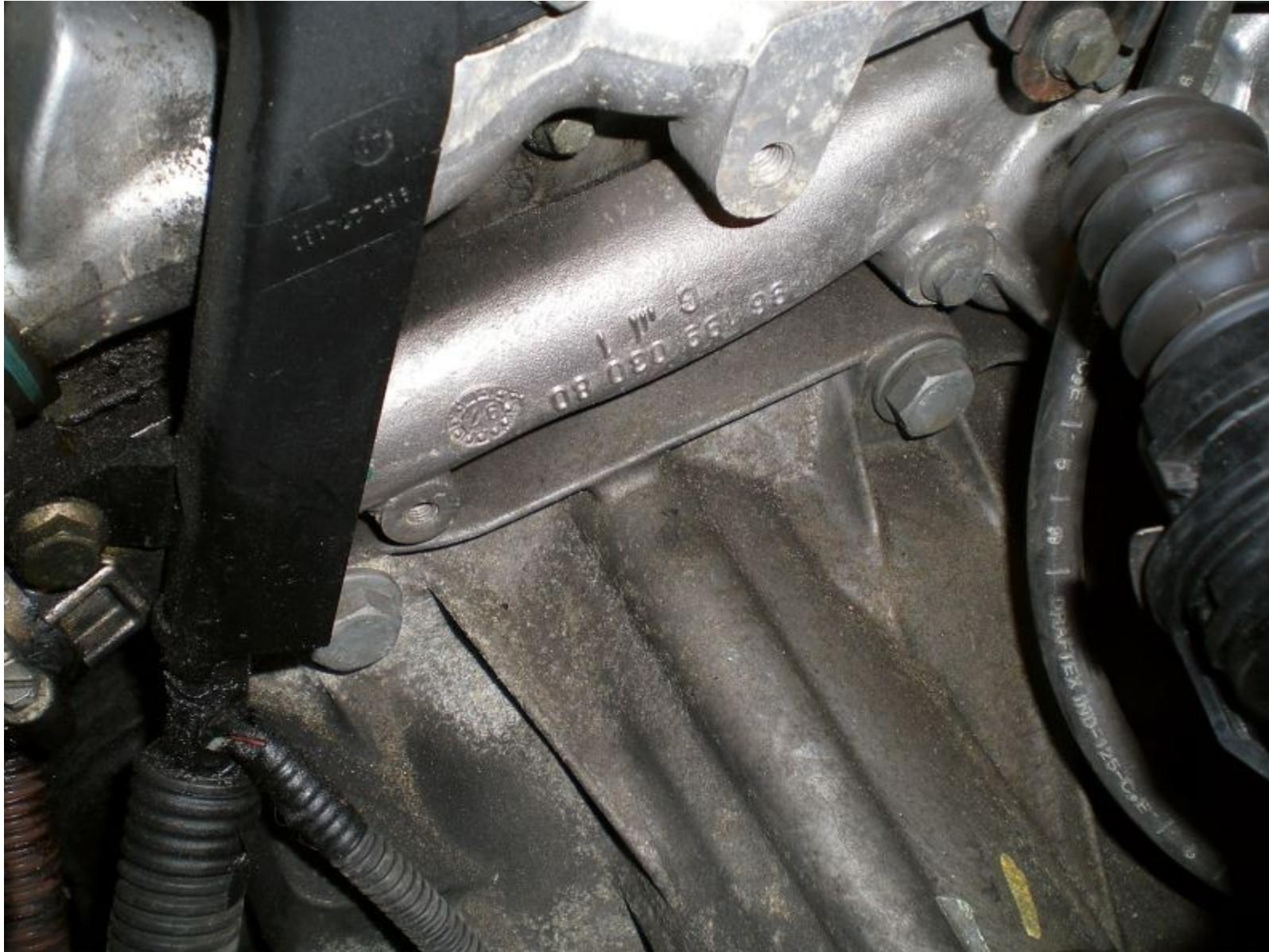
And one hard-to-reach one here in the centre of the picture. Don't forget there's also the backwards one underneath.
