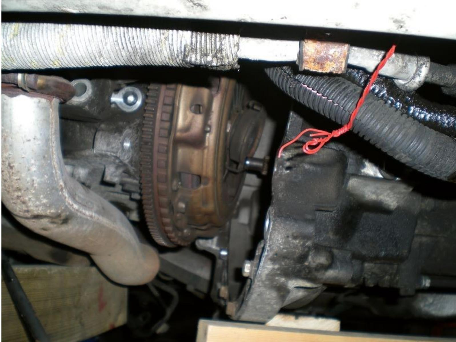
Expect the engine to want to rotate. This can lead to whoopsies like this. Also note that the holder for the Pin Of Evil makes a nice carrying handle if you wedge the handle of a breaker bar in it!!! Just be careful not to pull your brake wear cable like this. You can see how the gearbox has caused the jack to put a hole in my garage floor 🤪 It's HEAVY!!!
