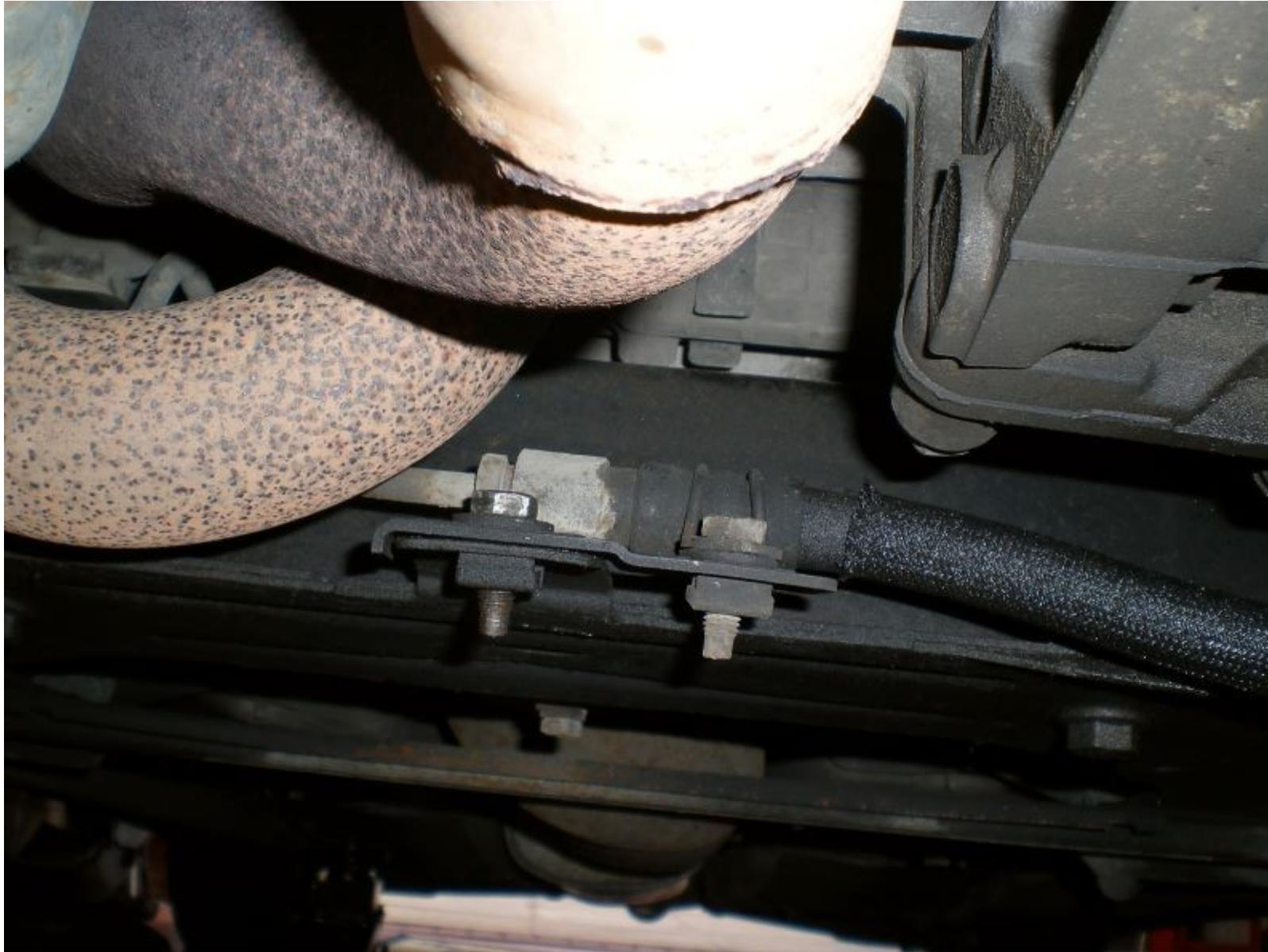
Unbolt the pipe from the gearbox too. There's 2 bolts to undo, the one at the front I've already removed in this picture.
