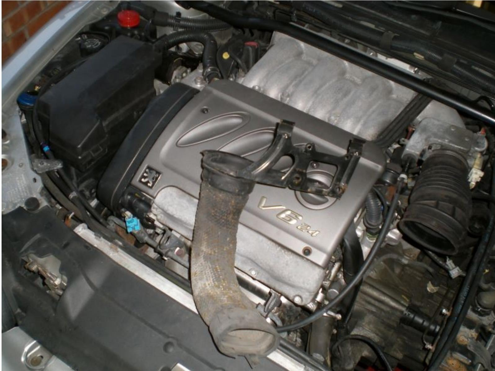
Not strictly required, but it can make the job easier if you remove the battery box. Use a ratchet with torx bit to undo the clip holding this aircon thing to it
