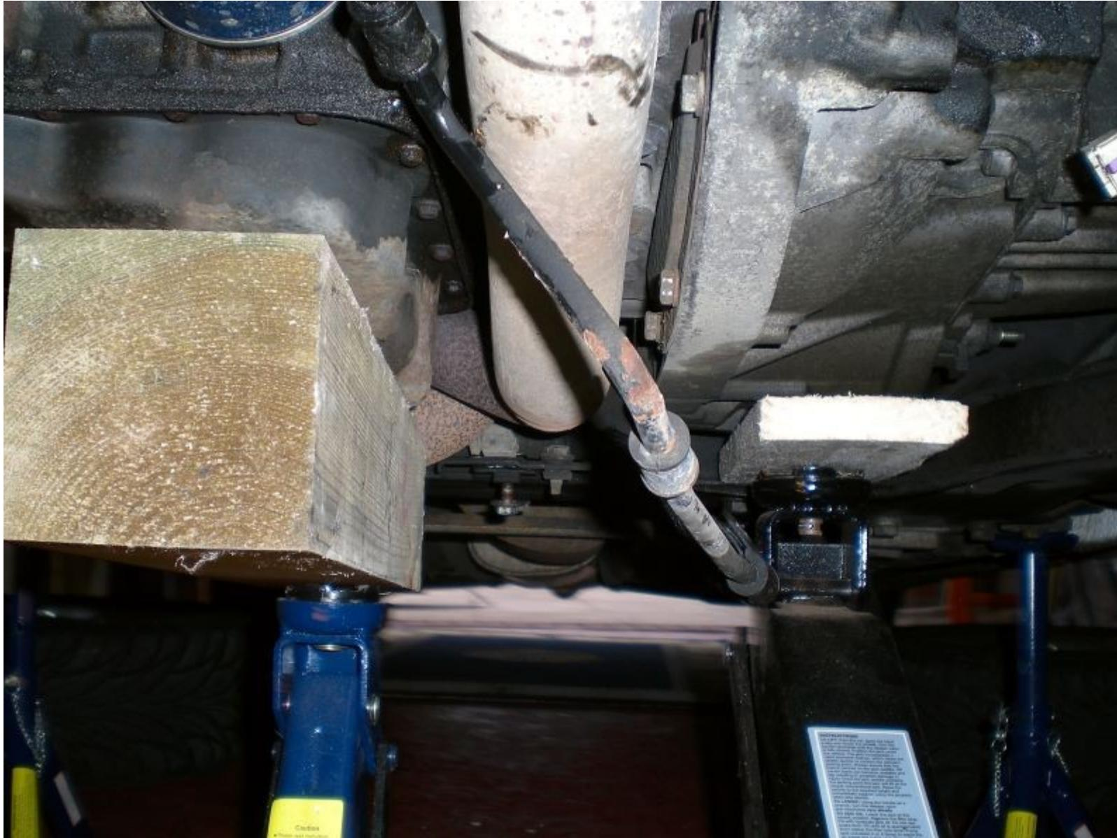
Up on top is the gearbox mounting. Take the large nut off then undo the 2 torx bolts to get the mount free.
