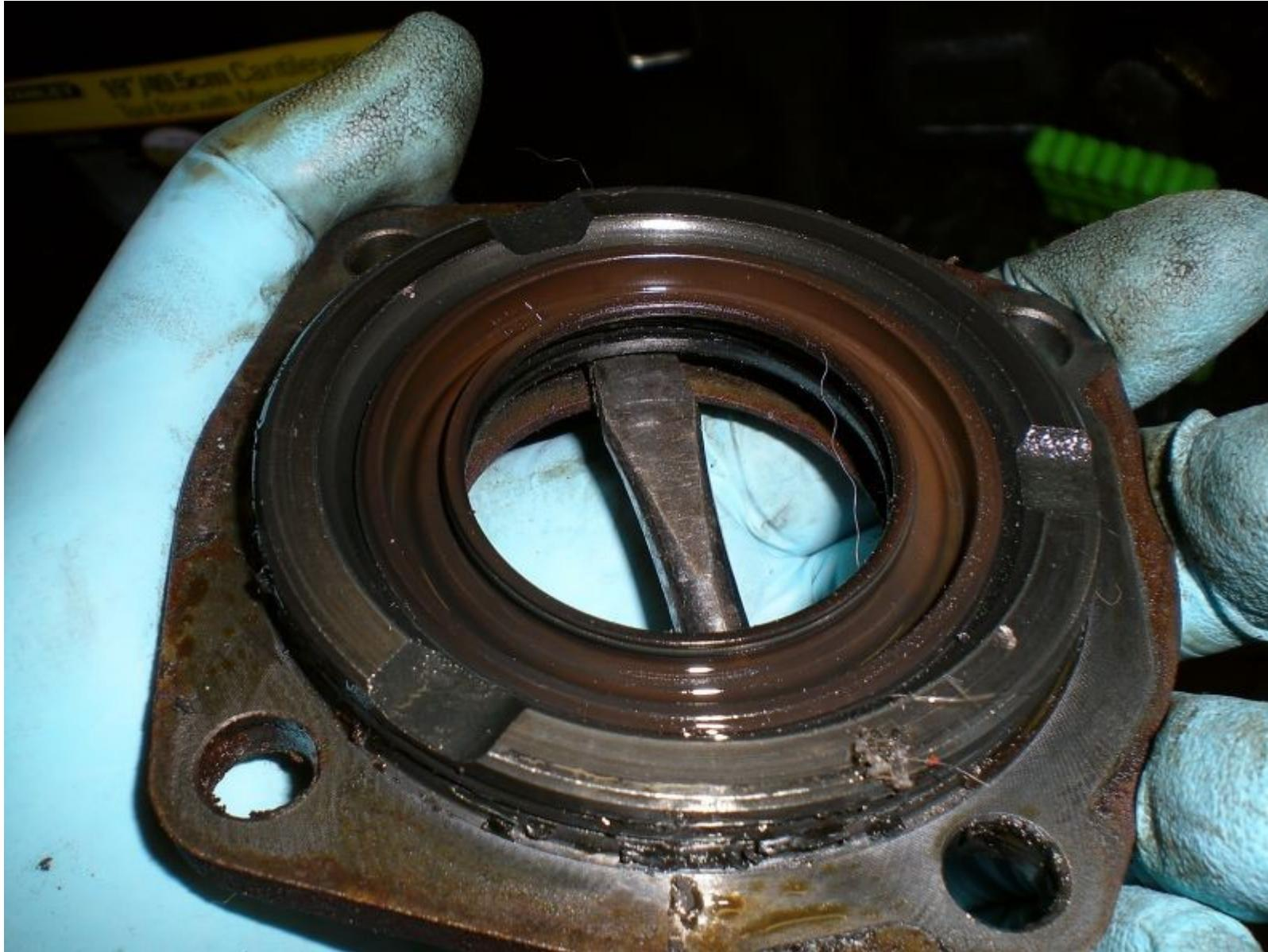
May as well clean up some of the muck from the gearbox while you can using some heavy duty engine degreaser. Note I've not gone mad with it, I've avoided seams and I've DEFINITELY avoided the gear selector's moving bits! You do not want degreaser inside your gearbox!
