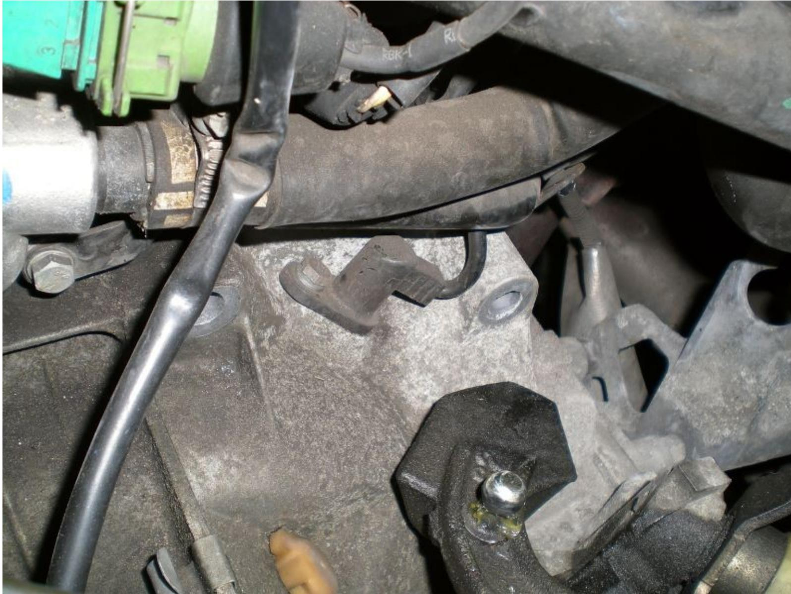
D9: The clutch slave cylinder has to come out now. This is not fun. Firstly free up as much of the pipework as you can. To remove it, you push it inwards and turn about 45 degrees anticlockwise. As you can see, I bent my pipe a bit 😞 Alternatively you can pull the steel clip that's holding the pipe in half-out and pull the pipe out. It'll be VERY messy though, and brake fluid's evil stuff.
