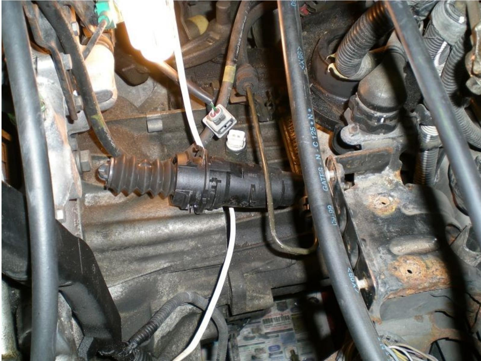
If you get back under the car and look behind the gearbox you should see something like this. Under the heat-resistant "bag" is the connector for the speed sensor. Pull him out.
