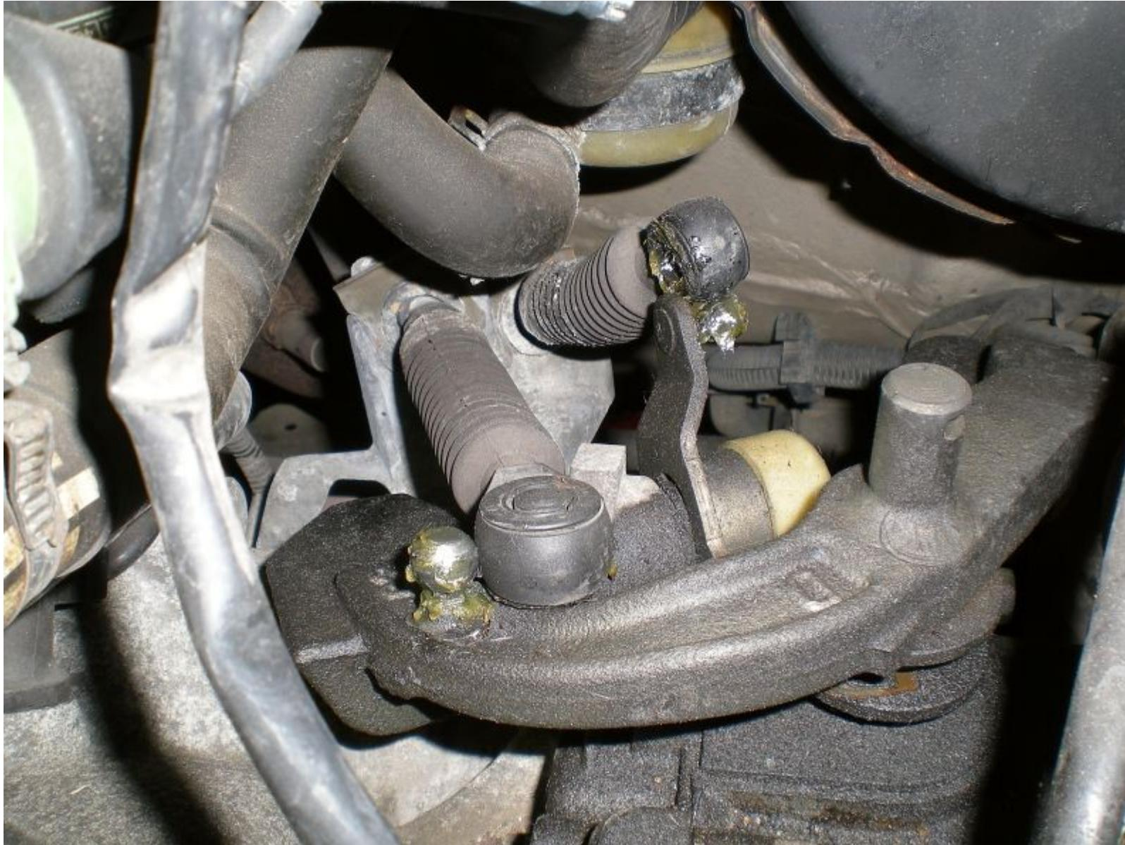
One 10mm bolt is all that's holding the flywheel sensor in. I strongly recommend you tie it up somewhere as it has a habit of falling around and catching on stuff
