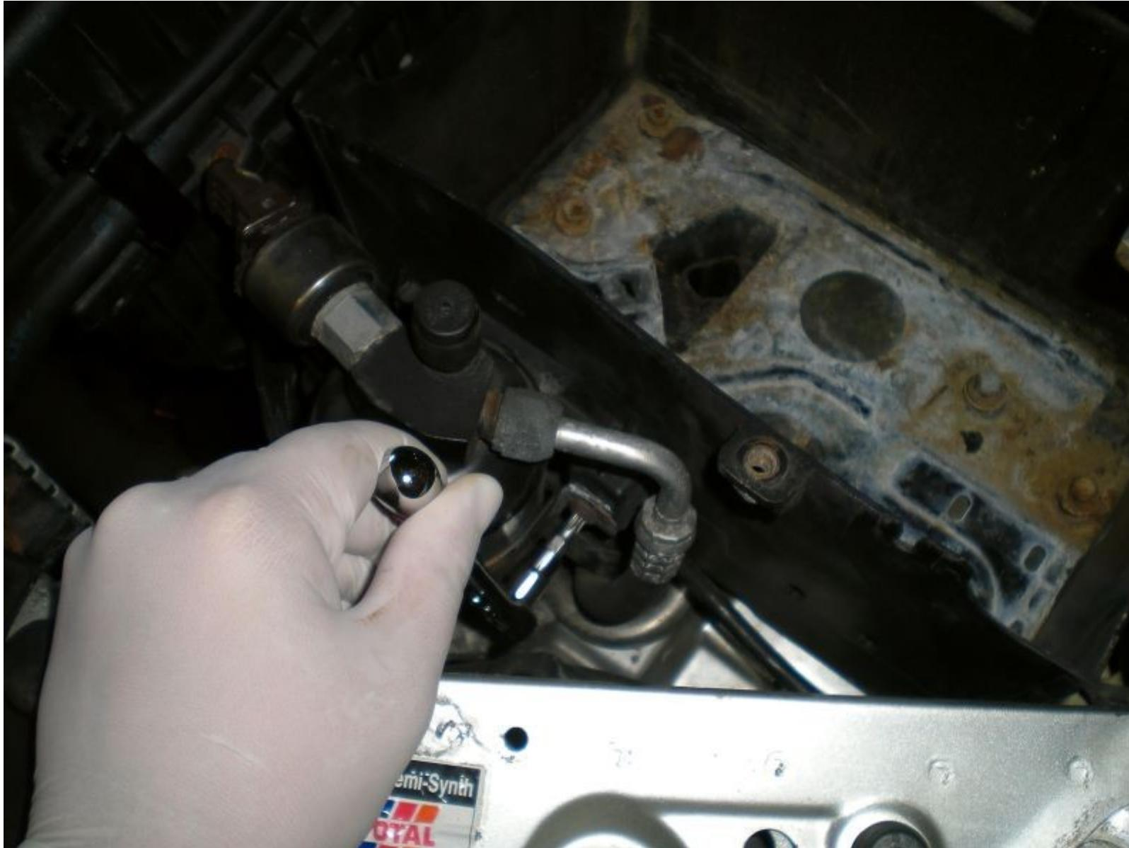
then pull the unit out slightly before sliding it to the right to unclip it. There's some wiring behind here you'll need to unclip
