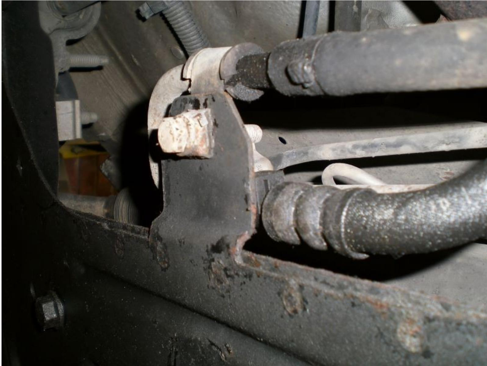
Remember the bolts under the steering rack? Undo them now. There's large ceramic washers between the rack and subframe, so catch these before they end up falling in your gob 😊
