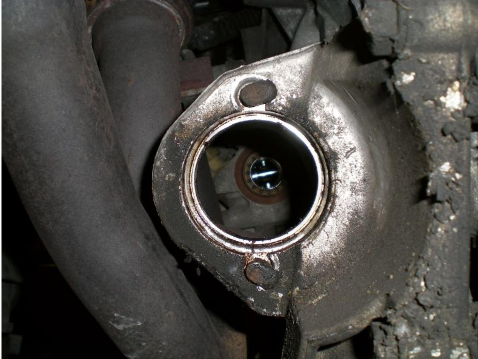
This is what you're fighting here, and without the subframe in the way a small 1/4" ratchet should have no problems getting in. Try not to damage the heat shield. It may be an idea to order a new one first since it's pretty brittle, but I put my old one back on later with a few big washers...
