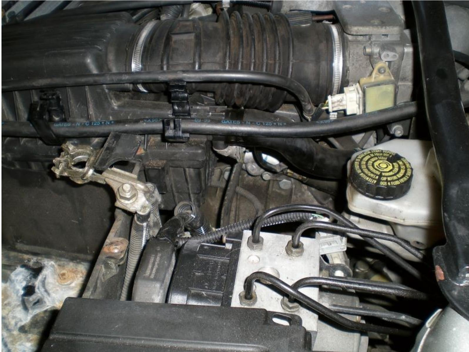
...and lift the air filter box out. There's 3 bolts holding this metal frame to the battery box. Remove them
