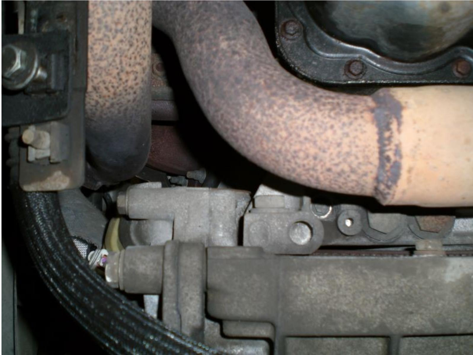
Now you want stuff to be supported. Don't jack stuff up directly, use a piece of wood to spread the load. You want to support the engine close to the exhaust pipe and the gearbox roughly where I'm showing here, but you want the jack pointing out of the wheelarch. Dunno why I had it like that in the picture
