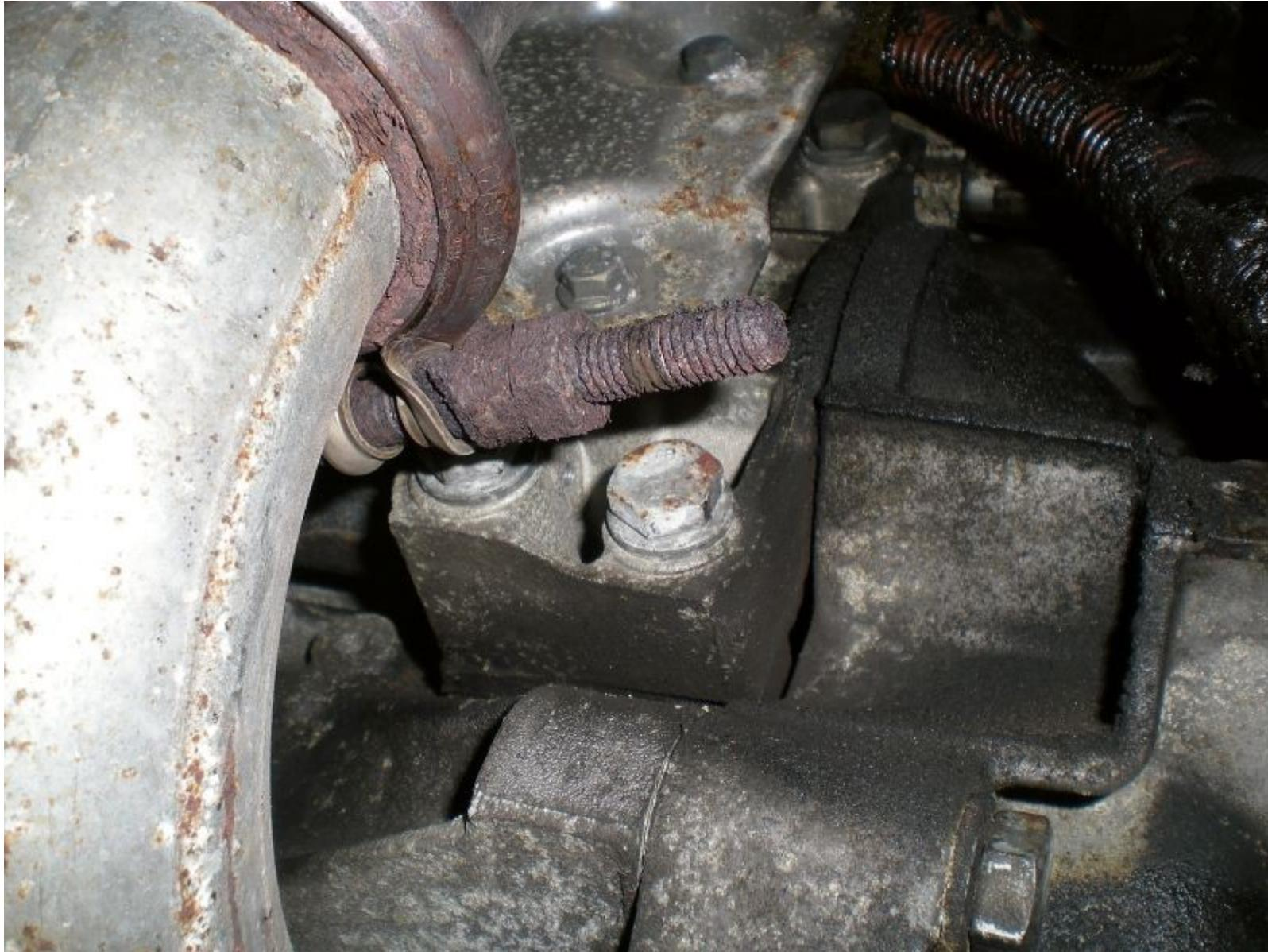
Without the shield, you can see the 3 bolts holding the starter in place - 1 at the top, 2 at the bottom.
