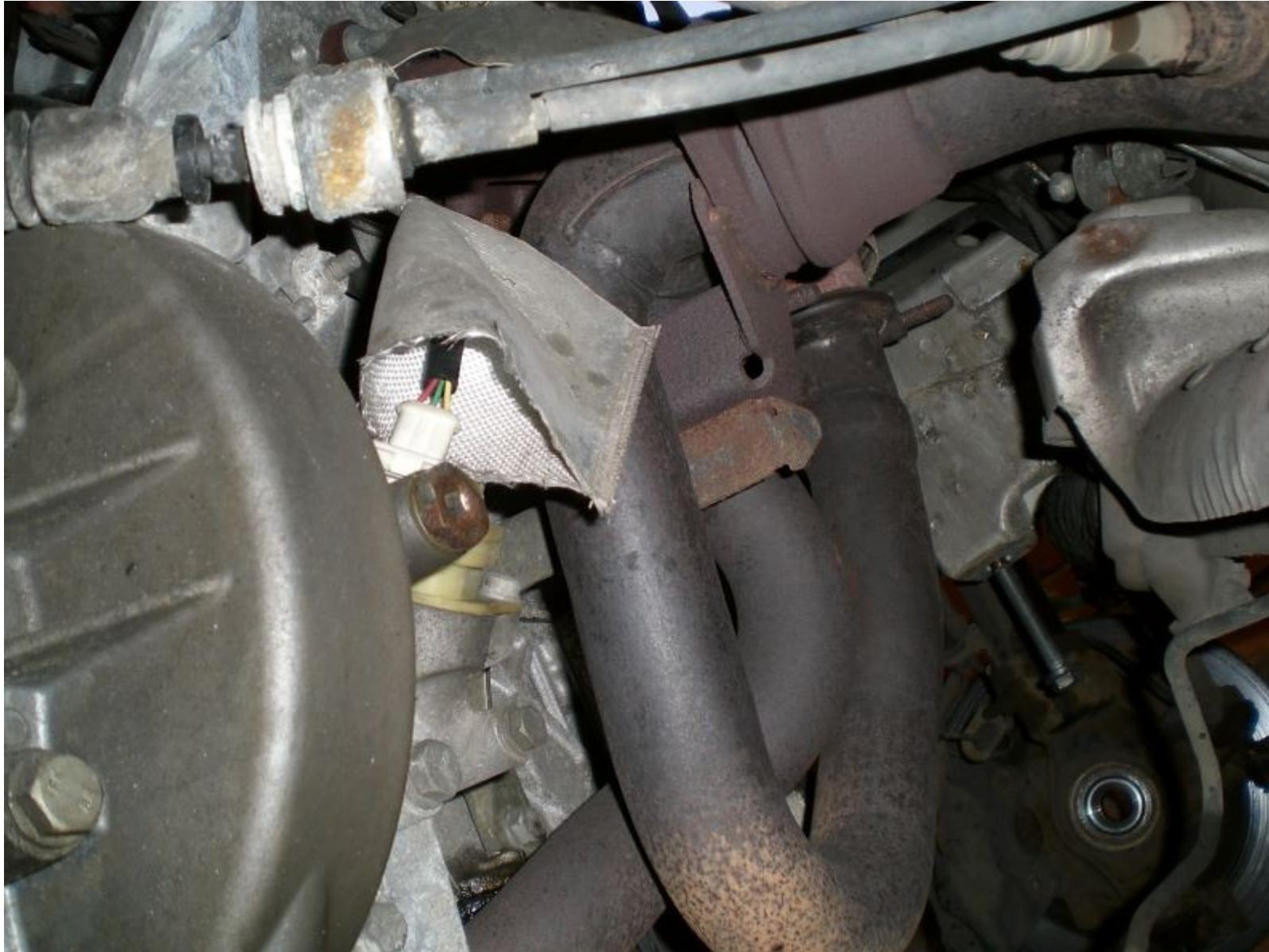
Up top, you should be able to see some wiring looms on a plate attached to the side of the gearbox by a big bolt right in the middle of this picture. This is the engine earth, and you'll want to clean up the plate, starter earth, and (once the box is out) the gearbox here.
