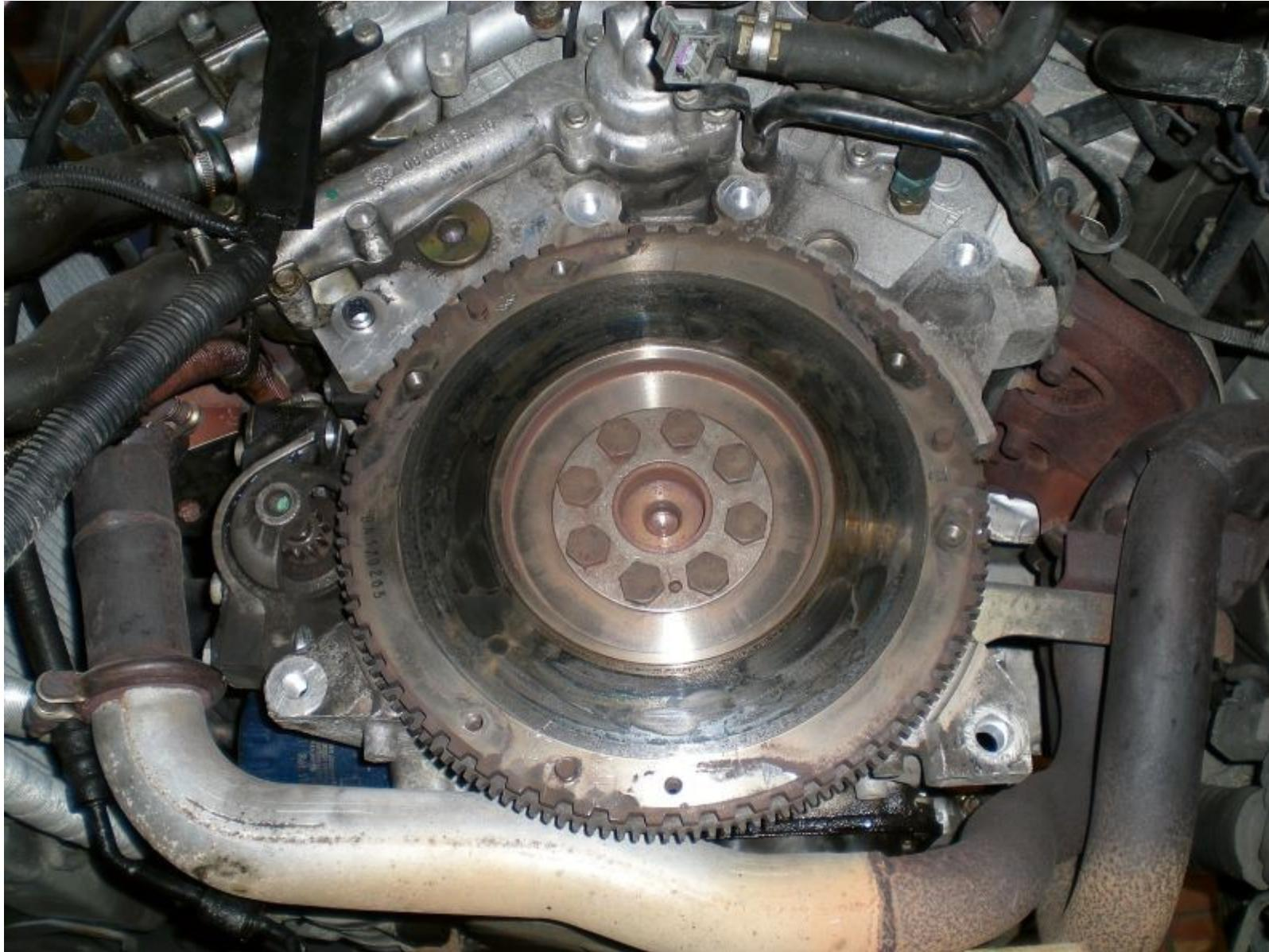
Fit the new clutch friction and pressure plates. The friction plate needs to be PERFECTLY in the centre. There's several ways you can do this, but be aware your average clutch alignment tool won't work.
