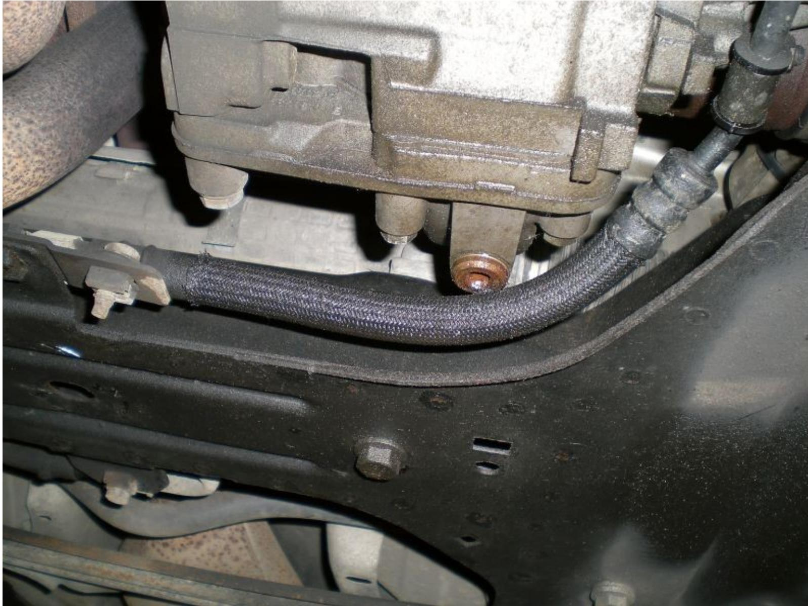
Here's the key you'll need to undo it with. 8mm square. I find it best to ignore the hole going through it and slap a ring spanner on the other end.
