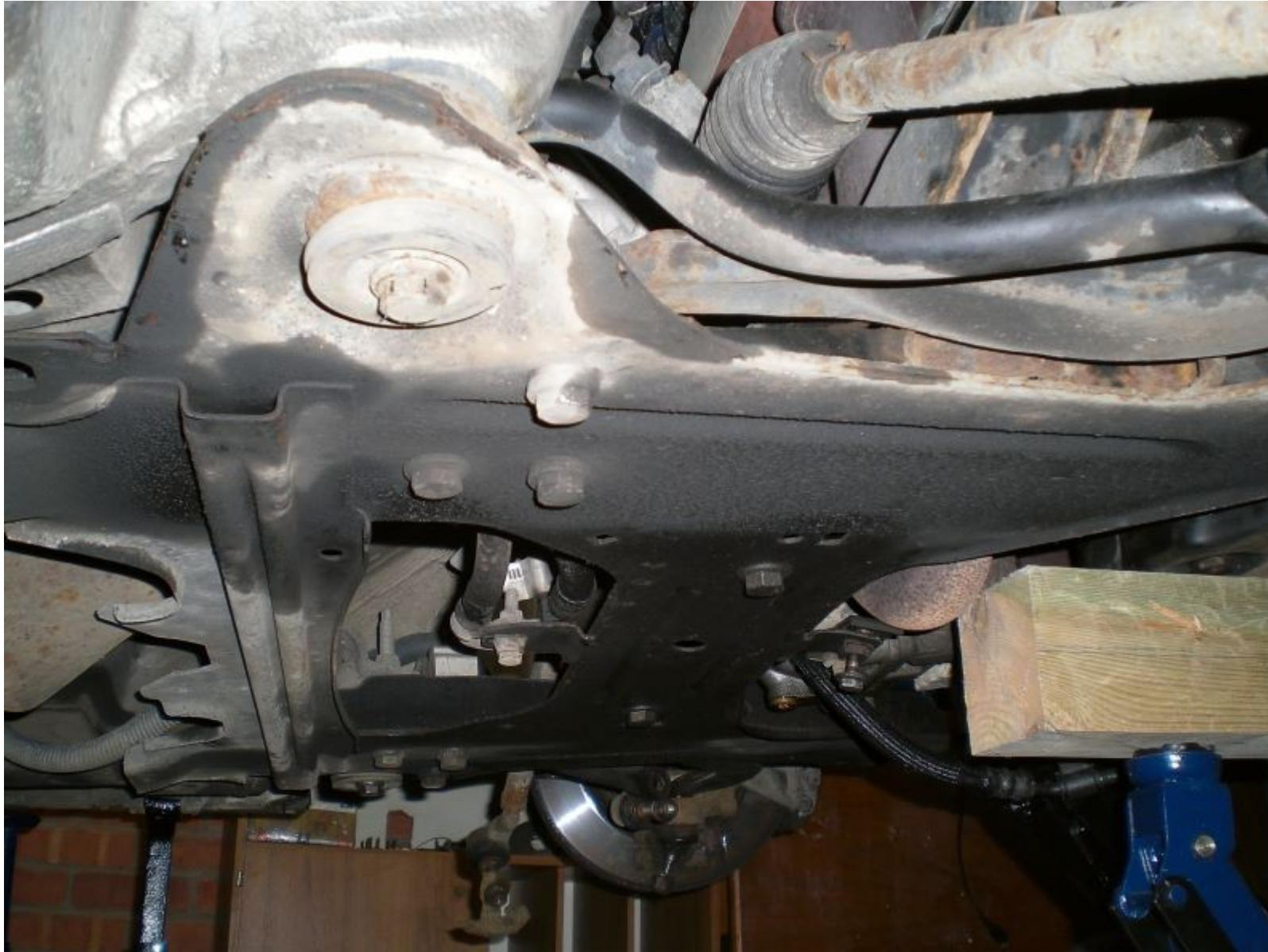
To the back of the main subframe bit (behind the steering rack) are these pipes held on by a nut+bolt. Undo to free the pipes.
