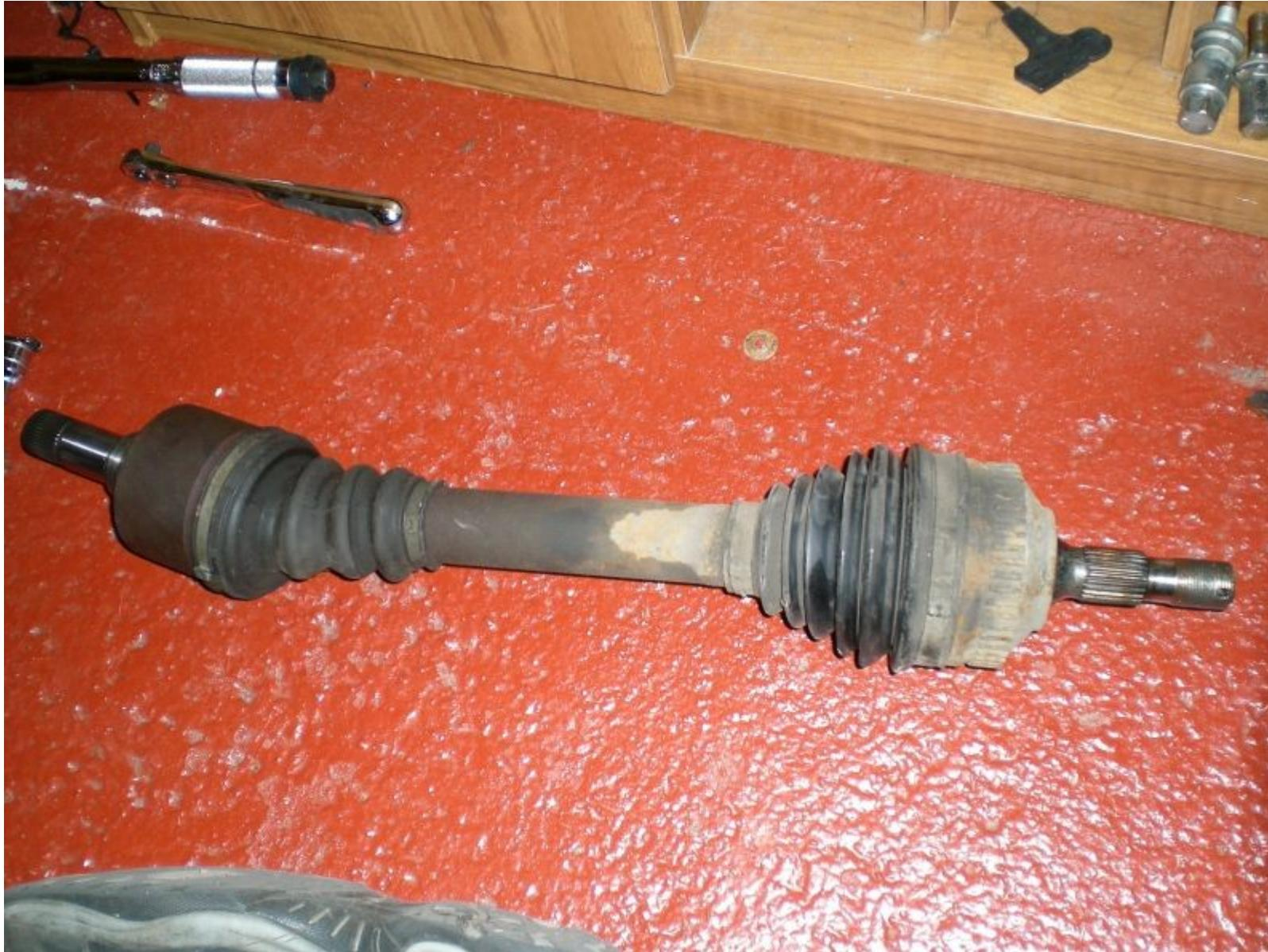
We can't remove the o/s driveshaft yet because it's held into the intermediate bearing (part of the lower engine mount), and the nuts to remove it are as good as inaccessible on the ES9J4 due to the 3 exhaust pipes in the way (may not be the case on the ES9J4S). So considering the subframe needs to come out to get the gearbox out, lets take it off.
