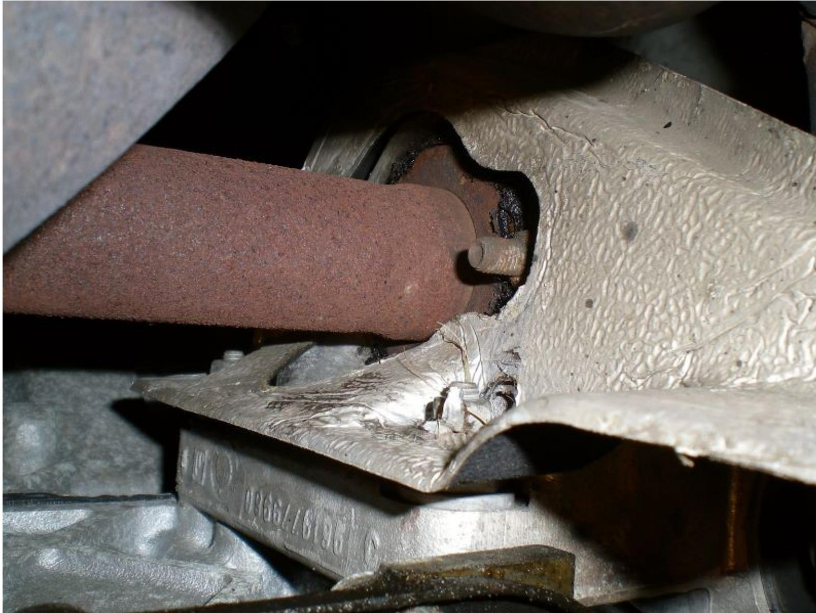
The o/s driveshaft should now pull out. Again, check for splits.
