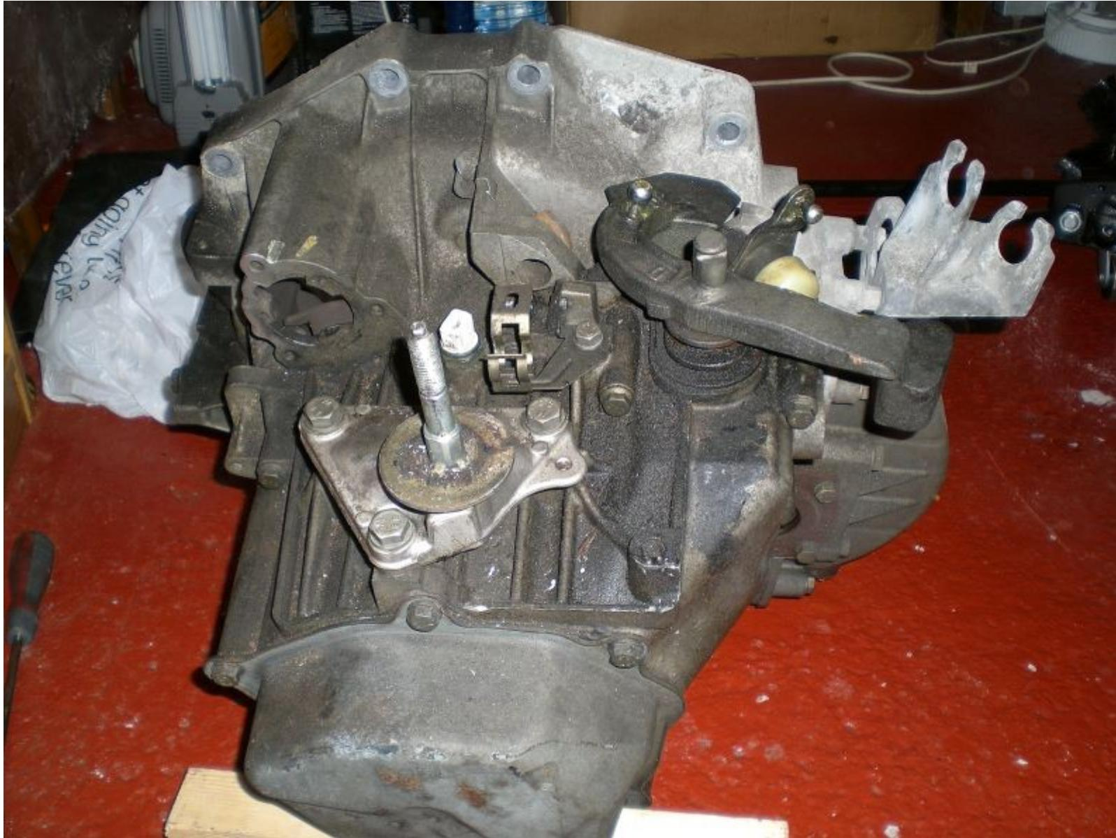
First job on the gearbox is to change this collar which the release bearing moves along.
