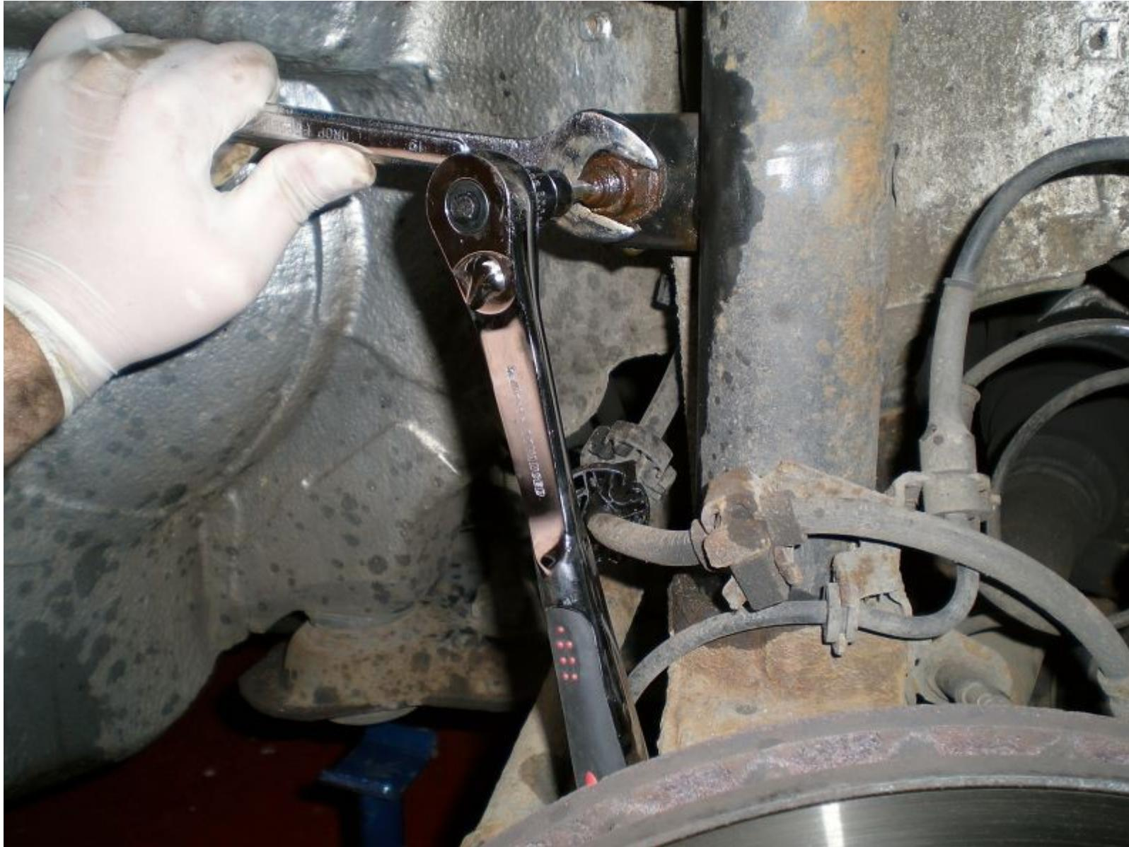
Now for the painful one 😬 You need to remove the nut from underneath the bottom ball joint (it's the type with plastic inside, so you'll need new ones to replace them) then wedge your ball joint splitter fork in there and use your biggest hammer to hit it like you've never hit anything before. I recommend you use earplugs here. When you've got the fork in enough, you can start to hit it up and down to help separate the wishbone from the hub carrier
