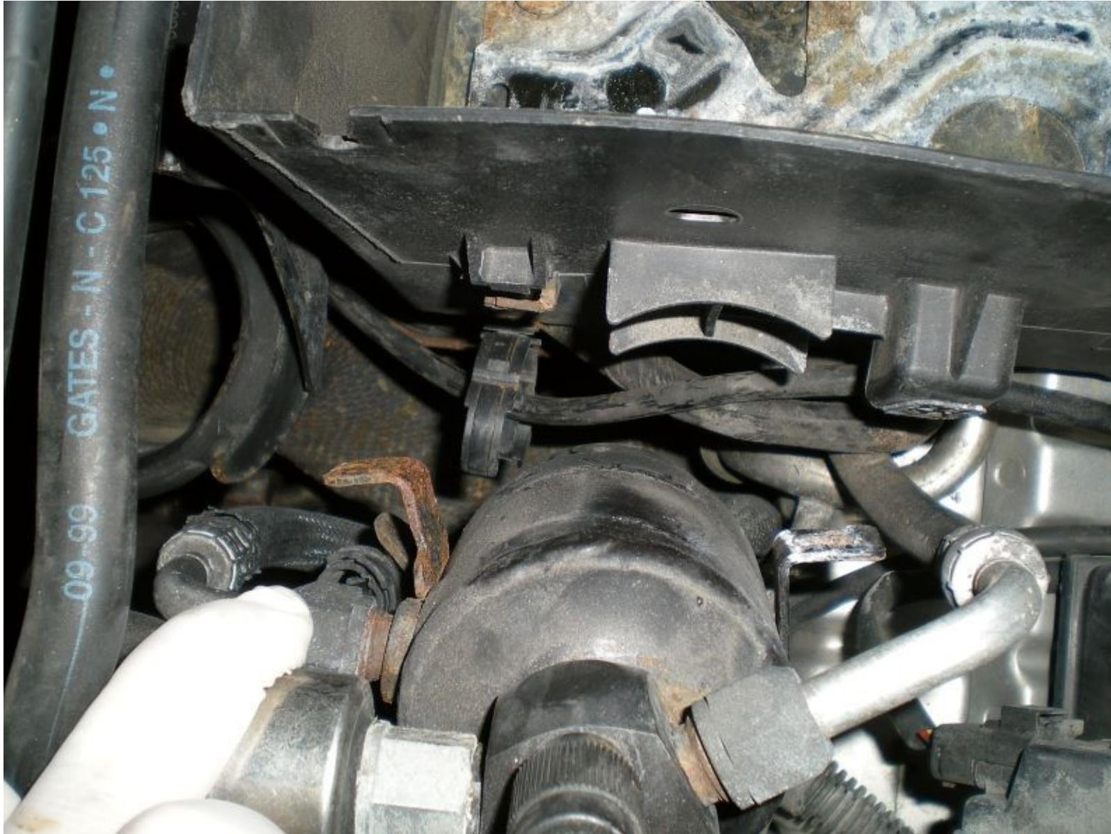
With the battery box out the way you can do some preventative maintenance if you want. Remove and clean up the main earth connection (shown to the right of the picture under the light connector), and check the wires are un-corroded and firmly in the battery clamp. I ended up cutting, stripping and re-attaching both wires.
