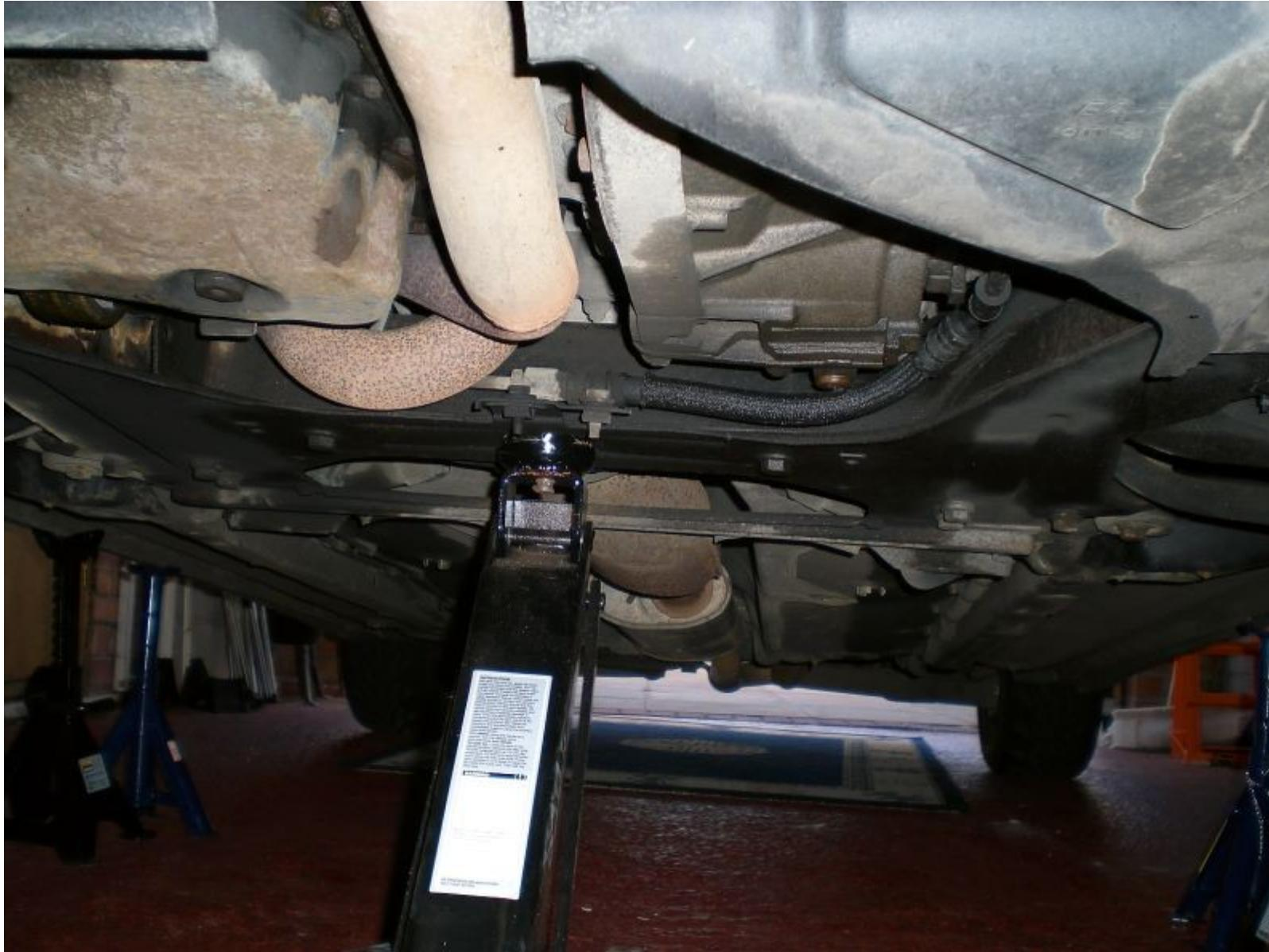
IMPORTANT!!!! Support the engine NOW with a bit of wood on a jack but don't raise the engine.
