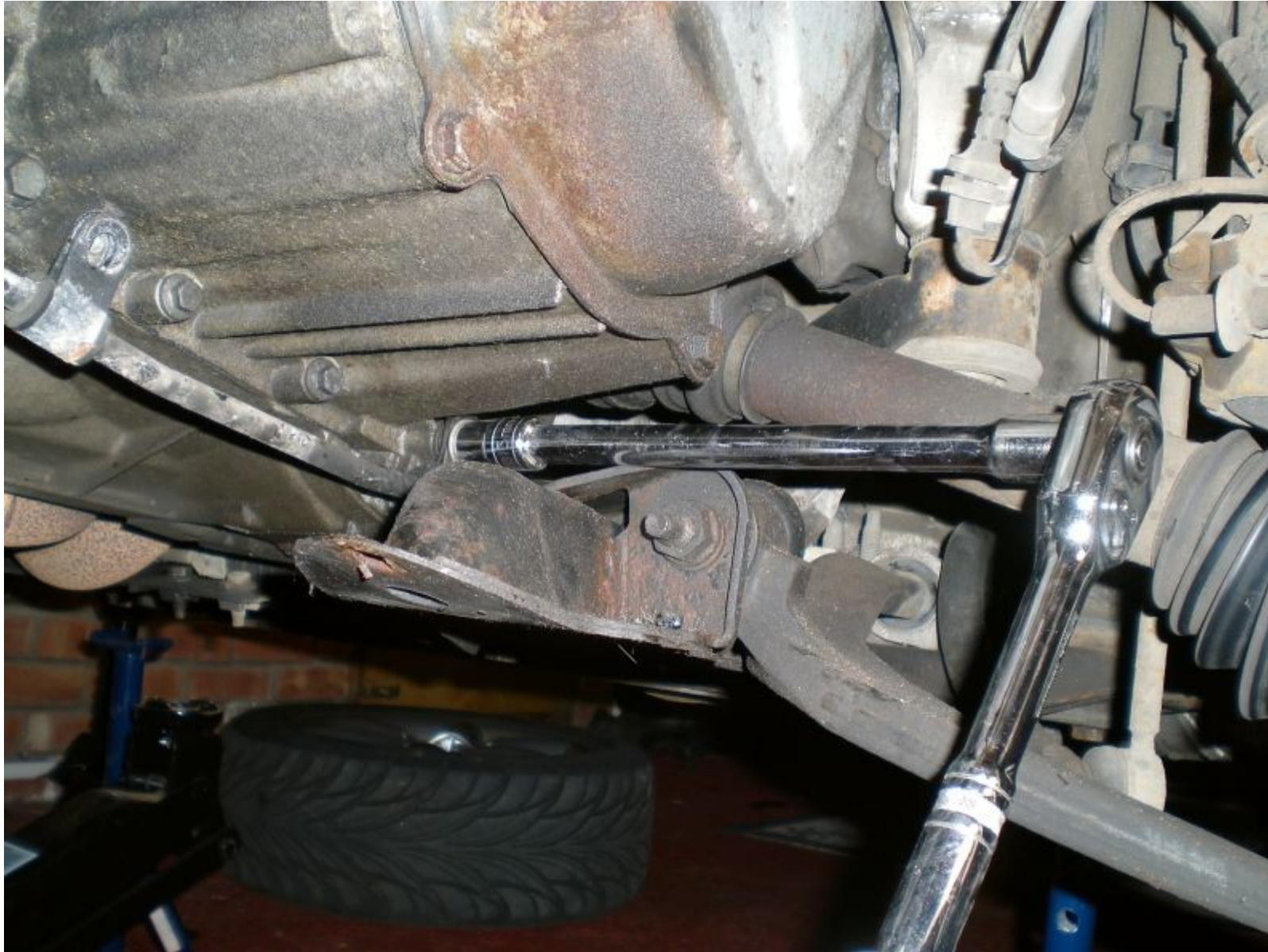
Here's the gearbox oil drain plug.
